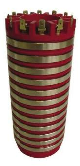
This range of slip rings has been designed to allow for greater adaptability and application of duty. They are suitable for slow and medium speed and are ideal for both power transmission up to 30 amps, and signal transmissions of all types. Best results are obtained when surfaces are plated with silver, gold or rhodium and used in conjunction with silver-graphite brushes, thus giving low contact resistance and low noise conditions.
